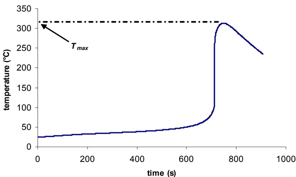
**Fig. 1.** Temperature profile recorded during a spontaneous FP (starting from the upper layer of the mixture) of a system B (see text) sample with 1.0 wt.-% Cab-O-Sil (sample 3B)
