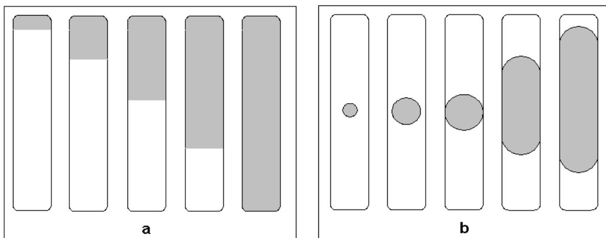
**Fig. 2.** Schematic representations of FP (unreacted mixture: white; polymer: grey). a) Typical descending front propagation (ignition is in the upper layer of the reacting mixture); b) 'spherical' front propagating from the centre of the mixture
