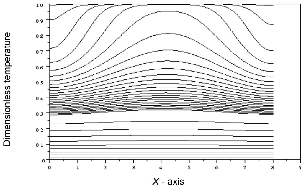
Fig. 16. Ignition and propagation of the reaction front for  $R = 5$  and  $\Lambda = 0.5$
