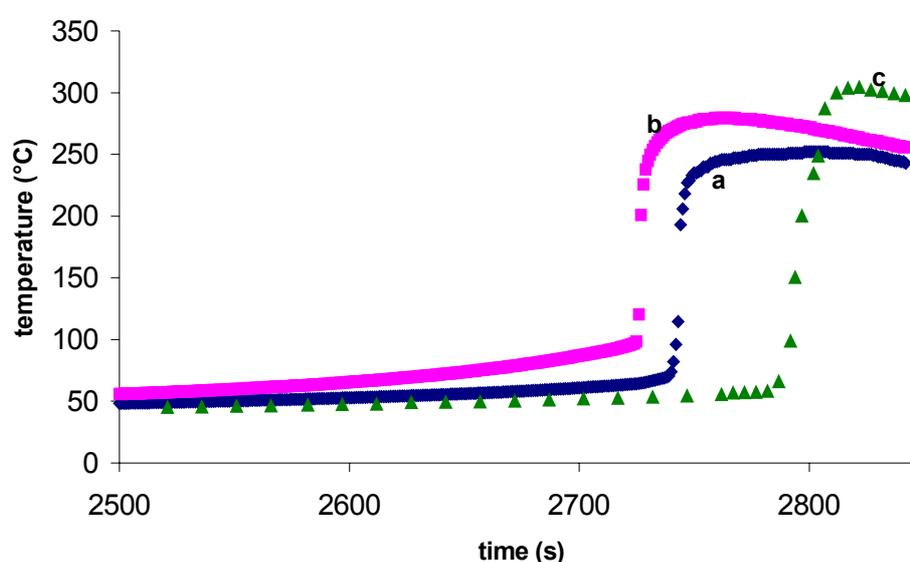
**Fig. 3.** Spontaneous FP profiles acquired during the phenomenon of self-ignition starting from the geometrical centre of the reacting mixture. Curves a, b and c are referred to data recorded at 1.0, 2.5 and 7.0 cm from the bottom of the tube, respectively (sample 2B)
