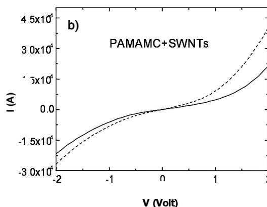
**Fig. 8:**  $I-V$  curves of (a) PAMAMC and (b) PAMAMC interacting with 1 wt% of SWNTs under on/off illumination steps in air (solid line sample without light, dashed line sample with light). The inset of Fig. 8 (a) shows the  $I-V$  curve of naphthalenediimide under on/off illumination steps in air.
