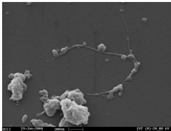
**Fig. 3:** SEM micrograph of the nanocomposite formed by PAMAMC + 1 wt% of SWNTs.
