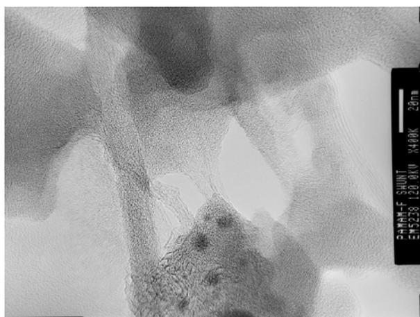
**Fig. 4:** TEM micrograph of the nanocomposite formed by PAMAMC + 1 wt% of SWNTs.
