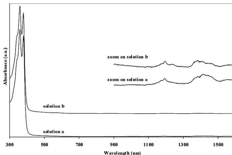
**Fig 2:** UV-Vis-NIR spectra of DMF soluble fractions of PAMAMC (solution a) and PAMAMC + 30wt% of SWNTs (solution b).
