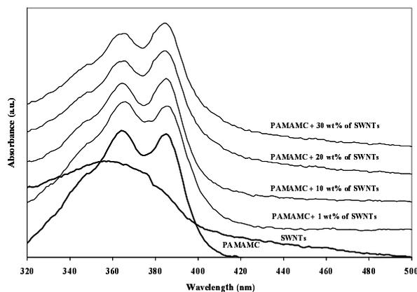
**Fig. 5:** UV-Vis spectra of PAMAMC, SWNTs and nanocomposites PAMAMC/SWNTs.
