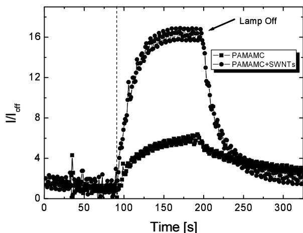
**Fig. 7:** Temporal photoelectrical resistance ( $I_{\text{off}}$  is the initial resistance of the sample with light off) response of PAMAMC and PAMAMC interacting with 1 wt% of SWNTs with on/off step illumination in air. At the time marked by the dashed vertical line, the sample was exposed to light.
