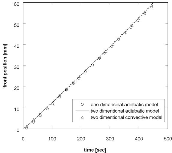
**Figure 7** Front advancement along the cylinder axis as a function of time: comparison of the results obtained from the one-dimensional adiabatic model and from the two-dimensional adiabatic and with convective boundaries, respectively.
