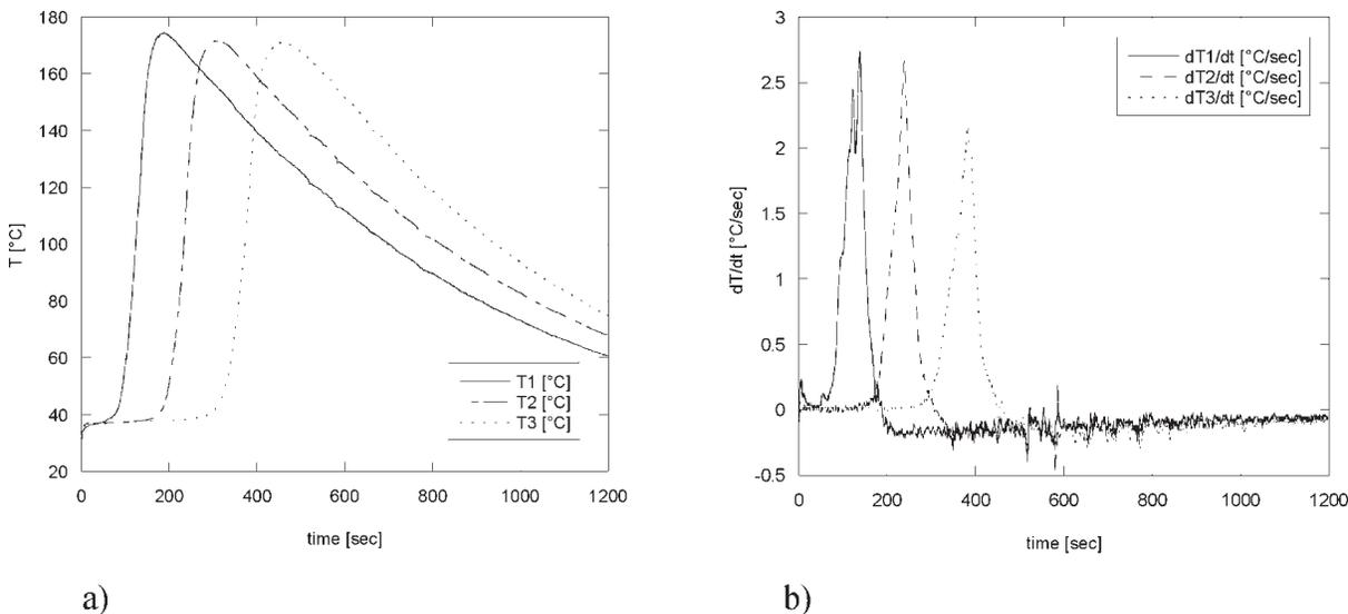
**Figure 1** (a) Temperature profiles of the three thermocouples fixed to the wall of the test tube reordered during the experiment. (b) Time derivative of the temperature profiles reordered from the three thermocouples fixed to the wall of the test tube.
