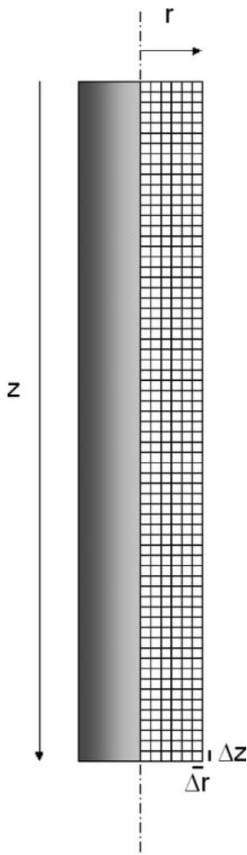
**Figure 9** Finite-difference grid considered for the two-dimensional model.
