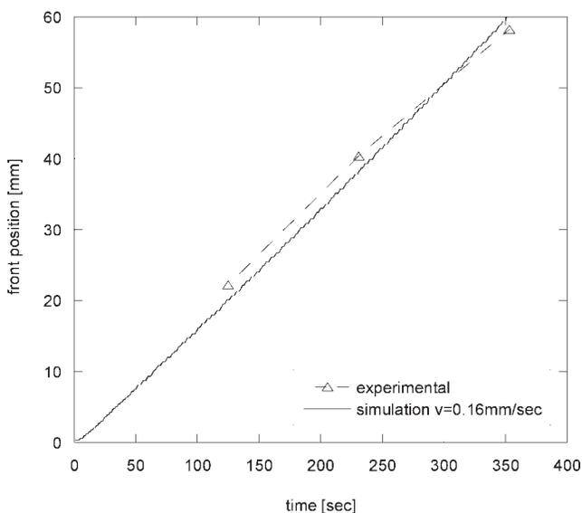
**Figure 2** Experimental results compared with the prediction of the model for front advancement along an axial direction. In the simulation, a  $C_p$  of  $2230 \text{ J kg}^{-1} \text{ K}^{-1}$  was used.
