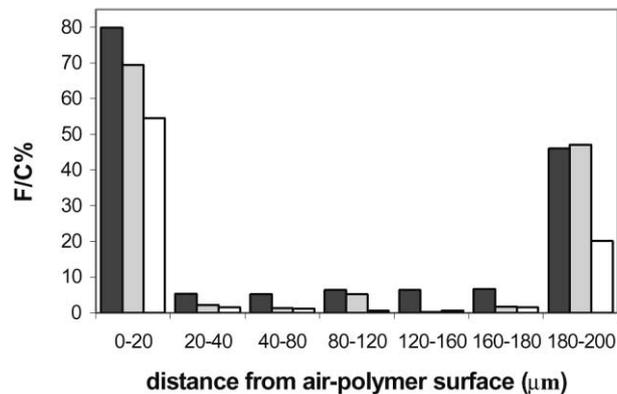
Fig. 7. The fluorine concentration, detected by EDX analysis, in the film sections across the (BMA-HEA-EA)-*g*-(PFPE-HMDI)/(BMA-HEA-EA) blends: (■) (20/80); (■) (10/90); (□) (5/95).
