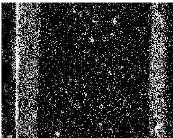
Fig. 6. The EDX mapping of the fluorine presence in the film section across the (BMA-HEA-EA)-*g*-(PFPE-HMDI)/(BMA-HEA-EA) (20/80) blend. The film has been solvent cast on PTFE dishes.
